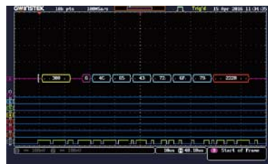
Decode by digital Channel
