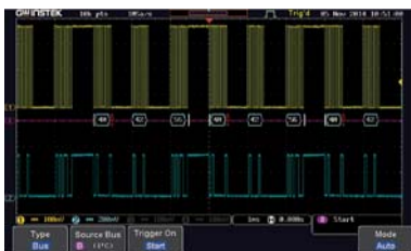
Decode by Analog Channel
