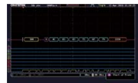
CAN Bus Trigger and Decode
